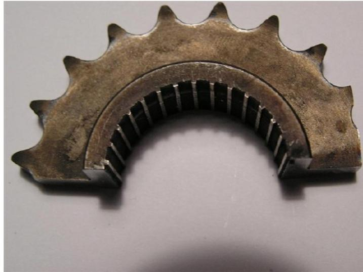
Figure 1a. A section of a failed Gen III camshaft drive sprocket. Photo by Bob Gervais. Downloaded from [2] with webmaster permission.
