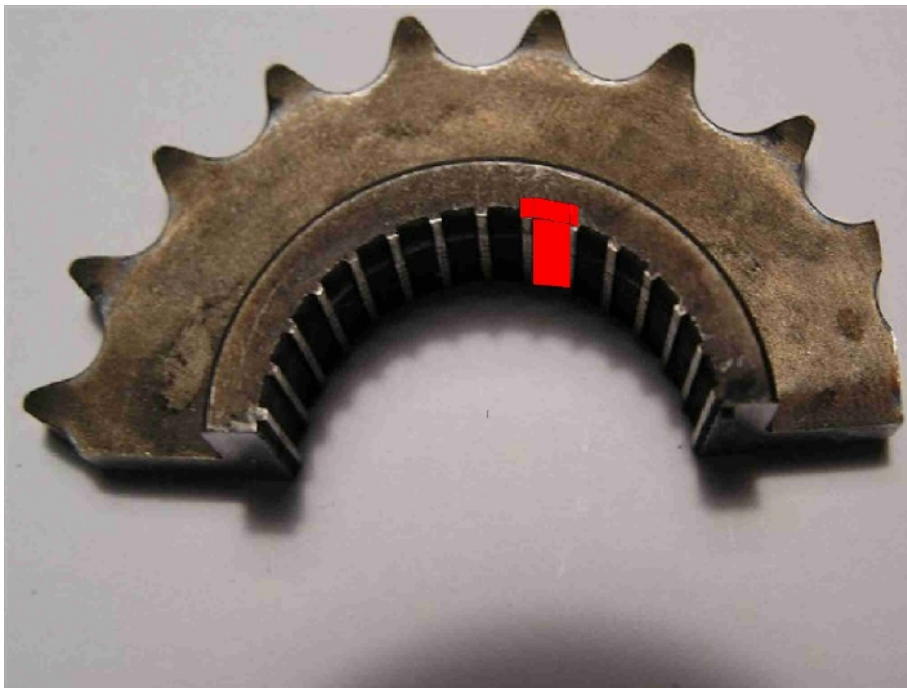
Figure 1. Gen III camshaft drive sprocket courtesy of Bob Gervais. Downloaded with permission from www.v8sho.com . The red detail of suggested adhesive void fill was added by B.C. Lamartine per a suggestion from Tim Wright. Adhesive fill must be replicated for all sprocket voids.
